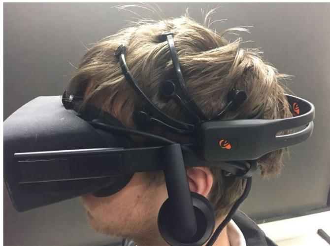
Figure 2: Demonstration of the experimental set-up showing the Oculus Rift VR glasses and Emotiv EPOC EEG headset.
