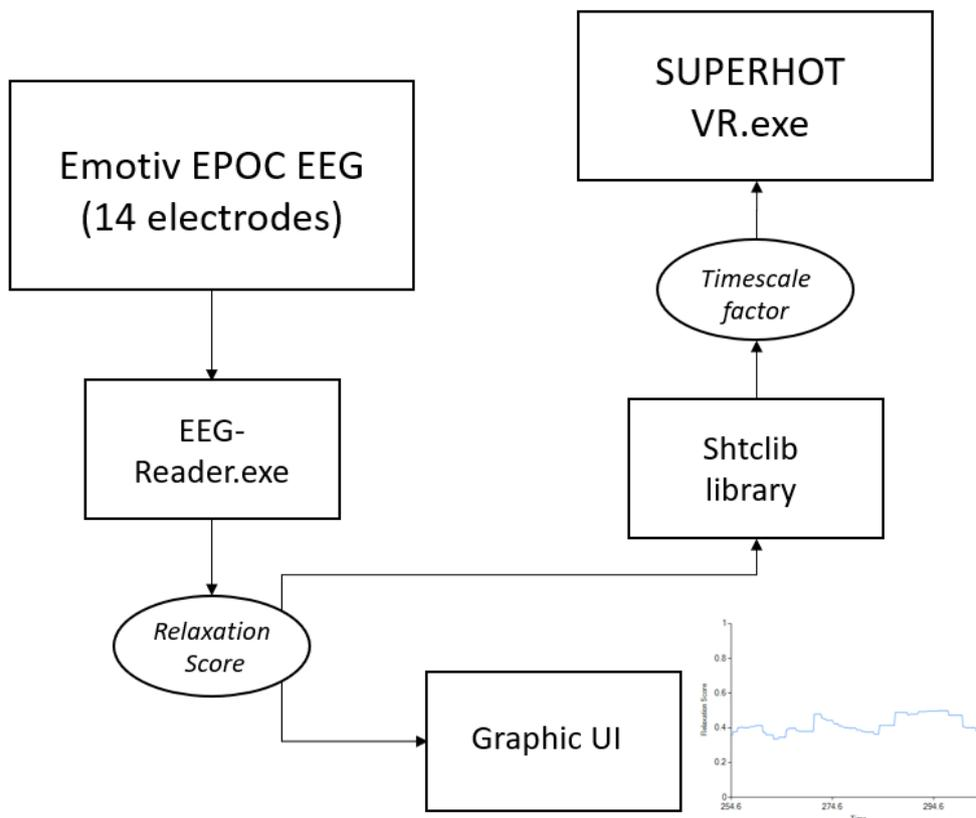
Figure 3: Visualization of the system developed for the experimental protocol. EEG-Reader.exe reads the current relaxation score from the Emotiv Xavier control suite. The relaxation is then fed into the Shtclib and converted into a time scaling variable, which is then called upon by the game.
