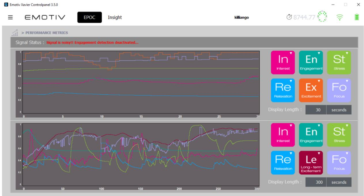
Figure 7: Screenshot of Emotiv Xavier Controlpanel demonstrating how the EEG was unable to calculate performance metrics due to noise. Even under perfect conditions (see top right) there were moments in which the signal was too noisy for an accurate calculation of relaxation.
